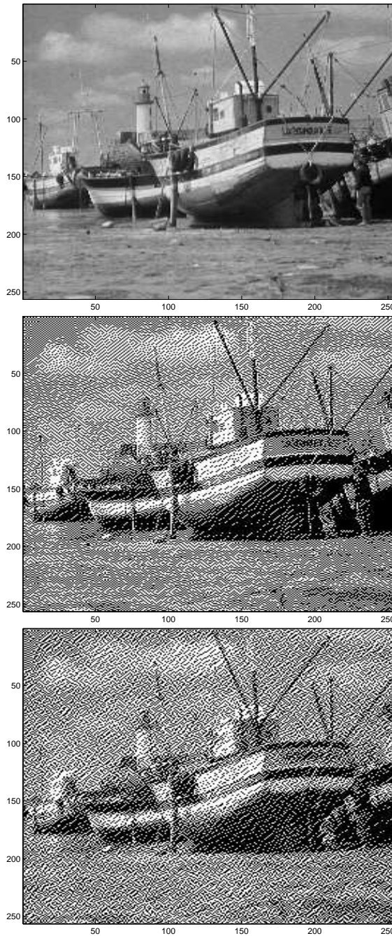
Figure 3.5: An example of halftoning a continuous gray-scale image. The top figure is a 256 \times 256 continuous gray scale image, the middle figure is a halftone of the top using (3.16), the bottom figure is a halftone of the top using (3.3).
